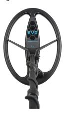
The EVO6000 comes with a **28 cm (11 inch)**, **17.5 kHz**, **elliptical search head** which is lightweight, great for finding coins and gives good depth. The elliptical shape creates a blade shaped field which gives a sharp signal when you sweep over a target. For more depth, for difficult sites or for special conditions other EVO search heads are available as **accessories**.
