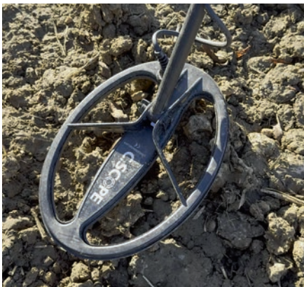
Fig.5. The 6MXi 20 x 28cm 2D elliptical coil.
